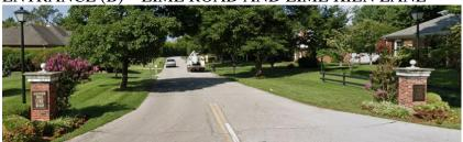
2 (TWO) EXISTING MOUNUMENT COLUMNS ON BOTH SIDES OF LIME ROAD TO BE REMOVED. NEW STRUCTURES TO BE CONSTRUCTED AS PROVIDED IN ARCHITECTURAL CONSTRUCTION DRAWING PLANS MATCHING ENTRANCE (A) COLUMNS FROM CITY MAYOR. ALL WASTE AND MATERIAL TO BE HAULED OFF SITE AND INCLUDED IN LUMP SUM PRICE FOR ENTRANCE (B). SITE MUST BE SECURED AT ALL TIMES DURING DEMOLITION AND CONSTRUCTION. UTILITES LOCATIONS WILL NEED TO CALLED IN AND MARKED BY CONTRACTOR PRIOR TO WORK BEGINNING.
